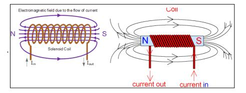
The magnetic field of an electromagnet decreases in strength as distance increases.
